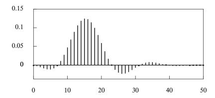
**Figure 19.** The coefficients from a finite-sample Butterworth filter of order n = 6 and with a cut-off frequency of  $\omega_c = \pi/8$ . The filter is appropriate to a sample of T = 51 points and the output  $x_t$  is at t = 15.
