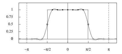
**Figure 10.** The frequency response of the 16-point wrapped filter defined over the interval  $[-\pi, \pi)$ . The values at the Fourier frequencies are marked by circles and dots. Note that, when the horizontal axis is wrapped around the circumference of the unit circle, the points at  $\pi$  and  $-\pi$  coincide. Therefore, only one of them is included in the interval.
