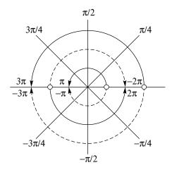
**Figure 1.** A diagram to illustrate the effects of aliasing in the process of sampling when there are frequencies beyond the Nyquist range  $[-\pi, \pi]$ , which defines the innermost circle. Frequencies on the outer circles are mapped onto the inner circle by following the radial lines, e.g.  $11\pi/4 \to 3\pi/4$  and  $3\pi/2 \to -\pi/2$  (The arcs with broken lines correspond to negative frequencies).
