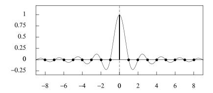
**Figure 2.** The scaling function  $\phi_0(t)$ . The function continues indefinitely in both directions.
