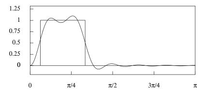
**Figure 9.** The rectangular frequency response of the ideal band pass filter defined on the interval  $[\pi/16, \pi/3]$ , together with the frequency response of the truncated filter of 25 coefficients.
