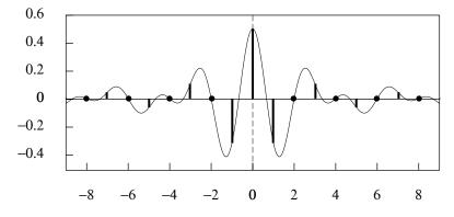
**Figure 4.** The wavelet function  $\psi_1(t) = \cos(\pi t)\phi_1(t)$ .
