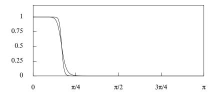
**Figure 15.** The frequency response function of the Butterworth filters of orders n = 6 and n = 12 with a nominal cut-off point of  $\pi/6$  radians (30°).
