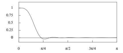
Figure 6. The frequency response function of the Henderson moving-average filter of 23 terms.
