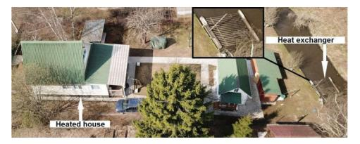
**Figure 2.** Aerial view of a heated house and a watercourse with a heat exchanger taken by from a quadcopter.
