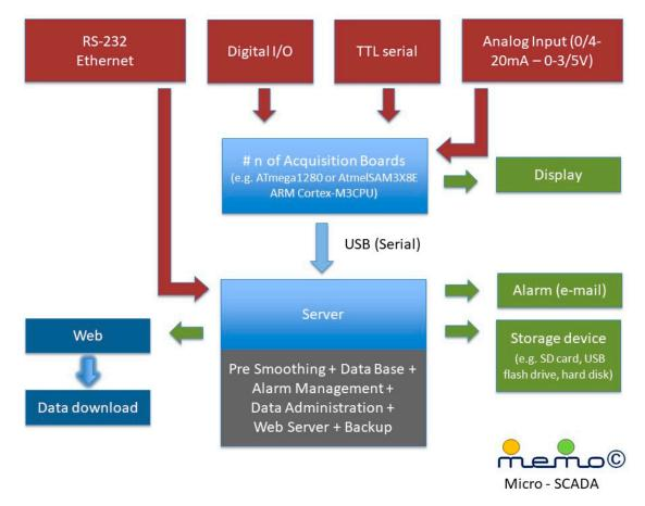
Figure 2. MEMO micro- supervisory control and data acquisition (SCADA).
