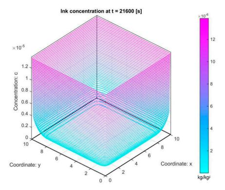
**Figure 7.** Migration of isopropylthioxanthone through PE packaging–isoconcentration profiles in milk with 3D model.
