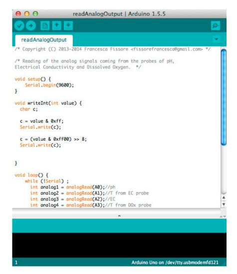
Figure A1. Read analog output.
