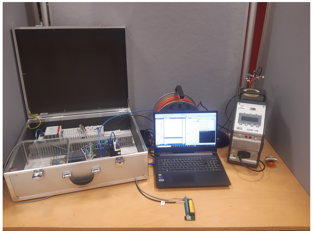
Figure 6. Experimental setup in real-world view. Left: PLC, center: notebook, front: TGW, right: temperature bath with temperature probes. The PLC is connected to the notebook via a direct Ethernet connection; the WiFi™ router for the gateway (GW) communication is not displayed. The two visible connections of the TGW correspond to the connected Pt100 temperature probe and a 24 VDC input signal to set the TGW up for internal processing instead of passing the signal (compare Section 2.1.1).
