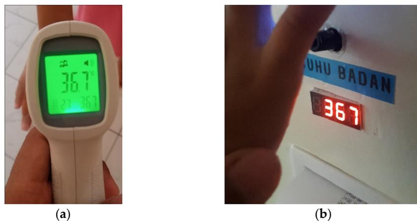
Figure 11. Body temperature measurement on: (a) Commercial Device; and (b) MLX90614-DCI Sensor.
