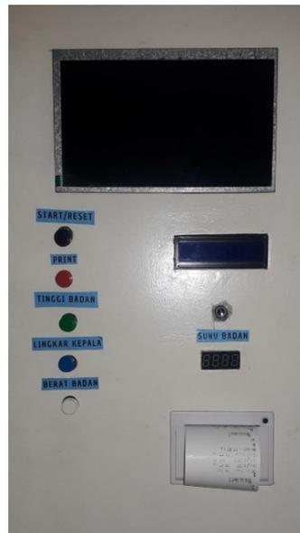
**Figure 2.** Control box of the anthropometric system and its components including push button. LCD 16 × 2, LCD 7 inch, seven segment display, temperature sensor, and thermal printer.
