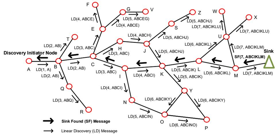
**Figure 2.** Propagation of an LD message in the LBD algorithm [39].
