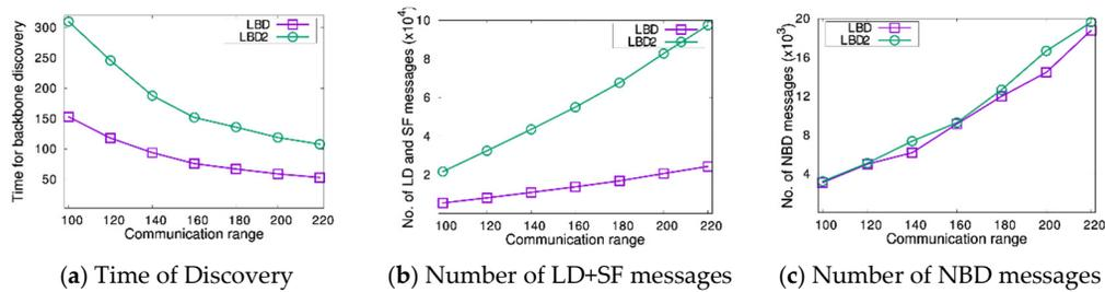
**Figure 7.** Performance results of the LBD and LBD2 algorithms as the communication range increased with the number of sensor nodes fixed at 1000. (a) Time of Discovery (b) Number of LD+SF messages (c) Number of NBD messages.
