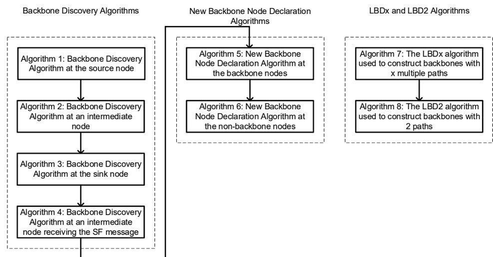
**Figure 4.** Flowchart showing the sequence of execution and relationship of the various algorithms.
