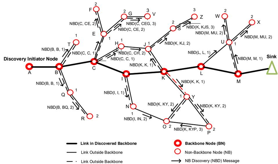
**Figure 3.** Propagation of the NBD message in the NBND algorithm [39].
