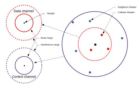
Figure 3. Basic architecture proposed for the RFID reader.
