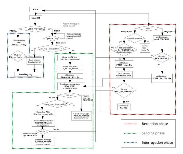
Figure 4. Proposed algorithm structure.
