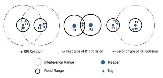
**Figure 2.** RFID collisions. (a) Reader-to-Reader Interference, (b) Reader-to-Tag Interference (1st type), (c) Reader-to-Tag Interference (2nd type).
