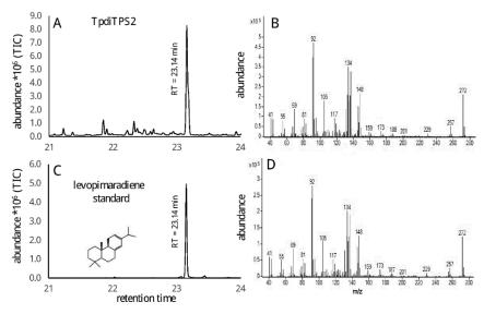
**Figure 6.** GC-MS analysis of levopimaradiene produced by TpdiTPS2 from normal-CDP. (**A**) = total ion chromatogram (TIC), (**B**) = mass spectrum of levopimaradiene, (**C**,**D**) = TIC and mass spectrum of an authentic standard of levopimaradiene produced by *Abies grandis* abietadiene synthase (AgAS) [63].
