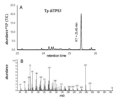
**Figure 7.** (**A**) = GC-MS analysis of copalol derived from geranylgeranyl diphosphate (GGDP) by TpdiTPS3, (**B**) = Mass spectrum of the chromatograph peak for TpdiTPS3.
