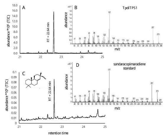
**Figure 4.** GC-MS analysis of sandaracopimaradiene produced by TpdiTPS1 synthase from normal- copalyl diphosphate (CDP); (**A**) = total ion chromatogram (TIC), (**B**) = mass spectrum of sandaracopimaradiene, (**C**,**D**) = TIC and mass spectrum of an authentic standard of sandaracopimaradiene produced by *Aspergillus niger* sandaracopimaradiene synthase (AnCPS-PS) [61].
