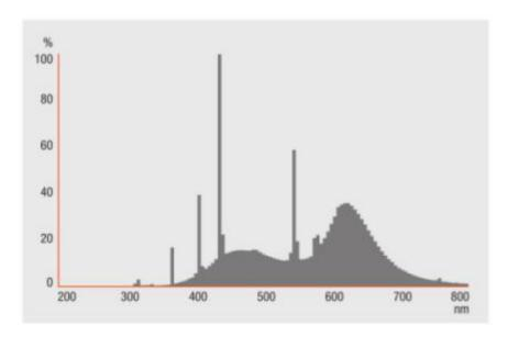
**Figure S1B** Spectrum of UV-B light emission from UV-B lamps (UVB GL20 SE, Sankyo Denki, Tokyo, Japan) provided by the Sankyo Denki company.
