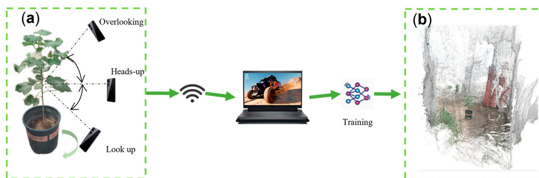
Figure 2. Data acquisition and nerf reconstruction. (a) Data acquisition. (b) Reconstruction results.
