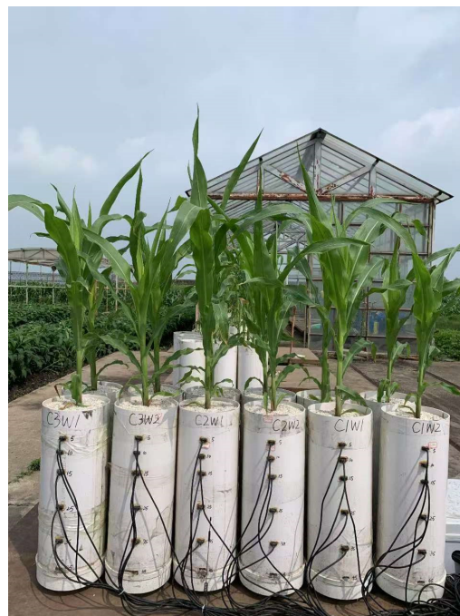
Figure 6. Experimental devices and soil water content monitoring.
