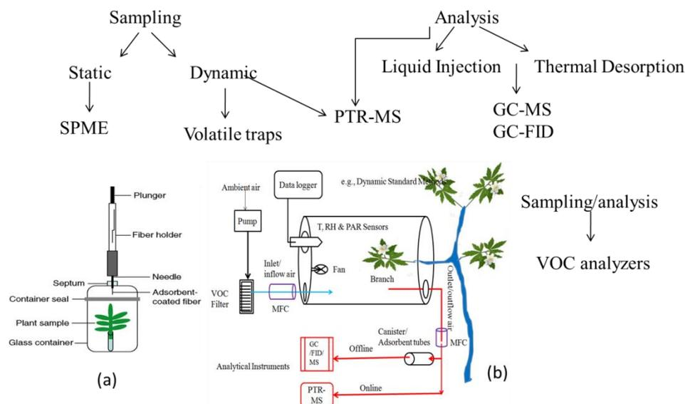
**Figure 2.** A schematic diagram of common analytical methods for determination of emission levels of monoterpenes from plants. (a) Static chamber method. (b) Dynamic enclosure chamber approach. (See text for abbreviations: Section 4).
