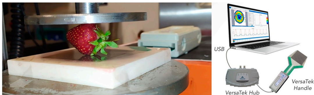
Figure 12. View of the compression test with a surface pressure measurement system (developed from www.tekscan.com (accessed on 29 May 2023)).
