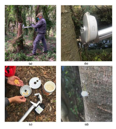
**Figure 3.** (a) Implanting a synthetic herbicide capsule into the stem of a *C. sinensis* plant using the InJecta<sup>®</sup> handheld device; (b) rotating drill bit (8 mm) creating a hole into the plant stem; (c) loading the magazine with synthetic herbicide capsules and polypropylene plugs; (d) polypropylene plug partially protruding from the implantation site of a treated *C. sinensis* plant.
