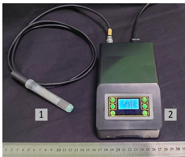
**Figure 2.** Photo of the “CAPKO-1” device for a CAP generation: 1—an output device with a silicone cap, on the surface of which a DBD CAP is created; 2—power supply unit and control of DBD CAP generation modes. The power consumption of the device is up to 40 W, and input voltage is 220–230 V.
