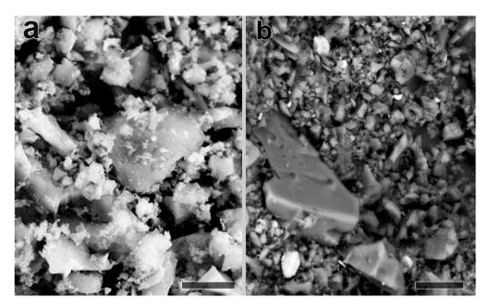
Figure 1. Surface microstructure of biochar (a) and granular activated carbon (b).
