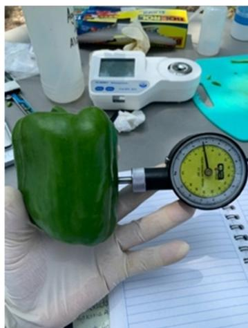
**Figure 4.** Use of manual penetrometer in bell pepper fruit.
