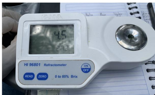
**Figure 5.** Use of digital refractometer for measurement of total soluble solids 4.8. Experimental design and statistical analysis.
