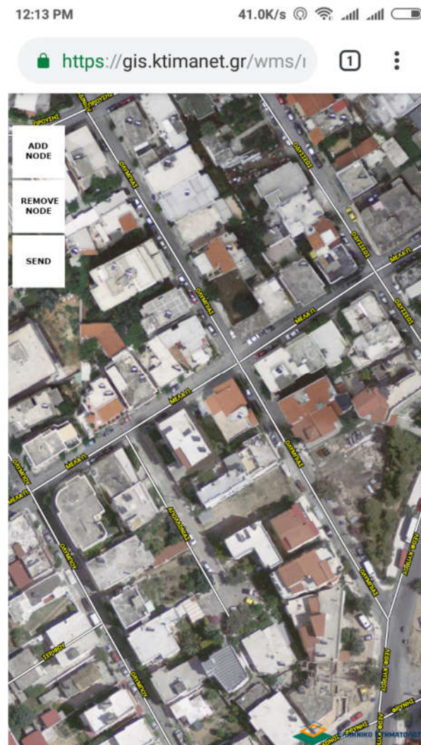
Figure 9. The web application tracks user position and gradually creates the parcel's boundary.
