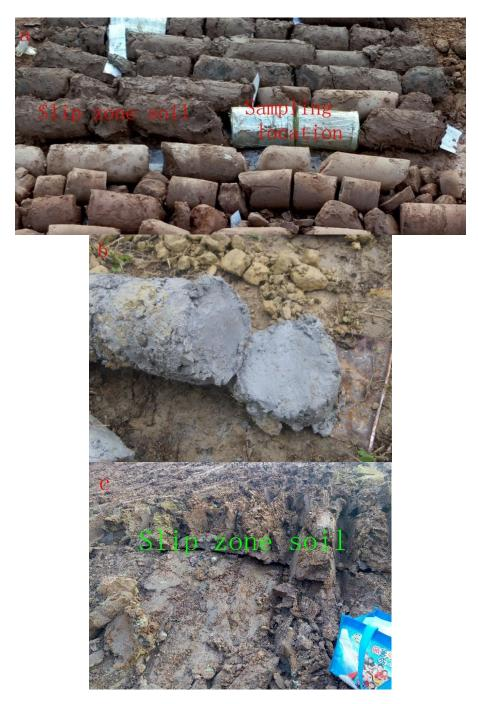
Figure 6. (a) ZK1-1 borehole sliding zone soil, (b) ZK2-2 drilling sliding surface soil, (c) sliding zone soil.
