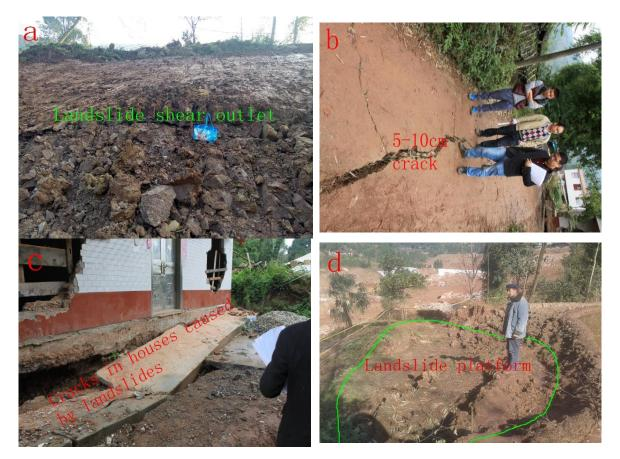
**Figure 4.** (a) Shear outlet in front of landslide, (b) rural road cracks on the back of the landslide, (c) cracks in the building foundation on the boundary of the landslide, (d) landslide platform on slide body.
