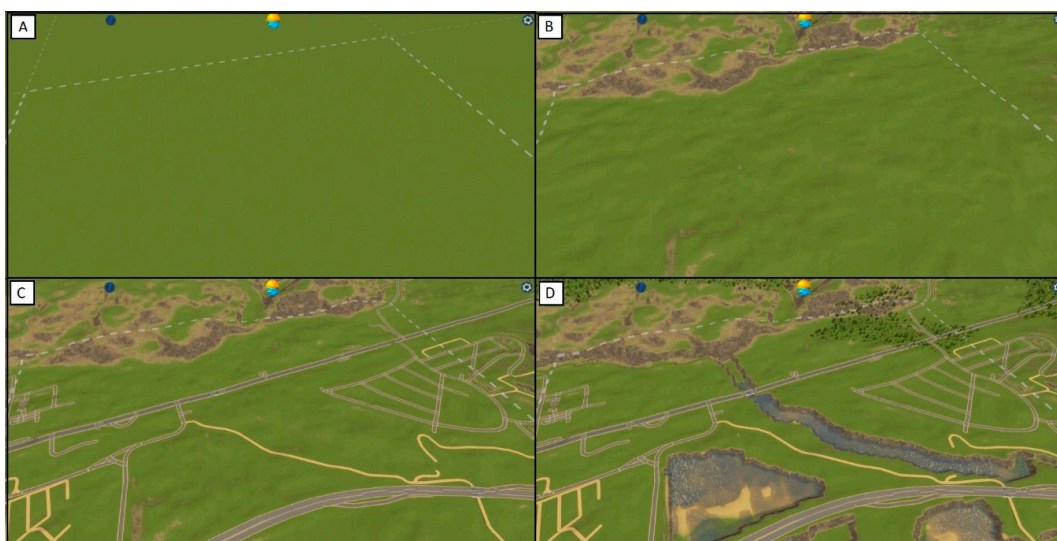
Figure 4. Creation of the base model of Svit from geographical data using the GeoSkylines methods. (A) An empty map after opening the map editor, (B) the map after uploading the terrain, (C) the map after generating the road network, and (D) the map after generating basins with water sources and tree coverage.
