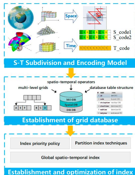
**Figure 2.** Workflow of the flight conflict detection algorithm based on the multilevel grid spatiotemporal index.
