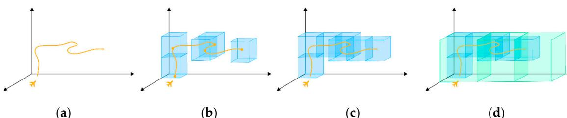
**Figure 4.** Path discretization. (a) flight path; (b) GeoSOT grid cells at key points along the flight path; (c) The path is discretized into higher level GeoSOT grids (smaller grid); (d) The path is discretized into lower level GeoSOT grids (bigger grid).
