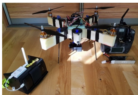
Figure 4. The designed UAV system (from the left: FPV receiver with cardboard, quadcopter with FPV system, mounted gimbal and GoPro camera, control equipment and LiPo battery).
