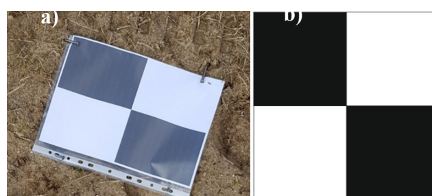
Figure 7. (a) Ground Control Point marked in the field with a white and black chessboard; (b) Project of the ground control point.
