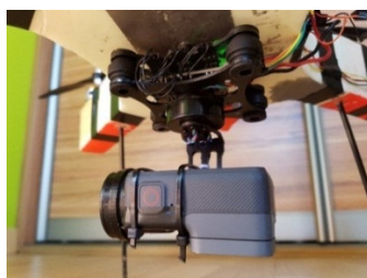
Figure 3. The method of attaching the three-axis gimbal together with the GoPro Hero 5 camera to the discussed multirotor – Unmanned Aerial Vehicle (UAV).
