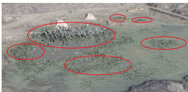
Figure 11. Errors on the point cloud created in areas flooded with water (marked in red ellipses).
