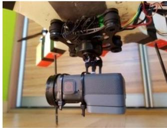
**Figure 3.** The method of attaching the three-axis gimbal together with the GoPro Hero 5 camera to the discussed multirotor–Unmanned Aerial Vehicle (UAV).
