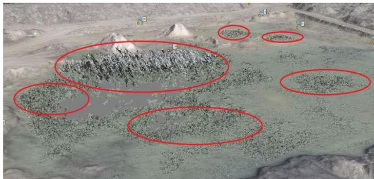
**Figure 11.** Errors on the point cloud created in areas flooded with water (marked in red ellipses).
