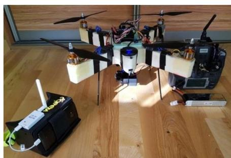
**Figure 4.** The designed UAV system (from the left: FPV receiver with cardboard, quadcopter with FPV system, mounted gimbal and GoPro camera, control equipment and LiPo battery).
