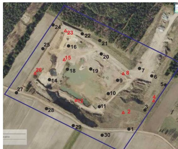
**Figure 8.** The arrangement of photogrammetric network points on the study site.
