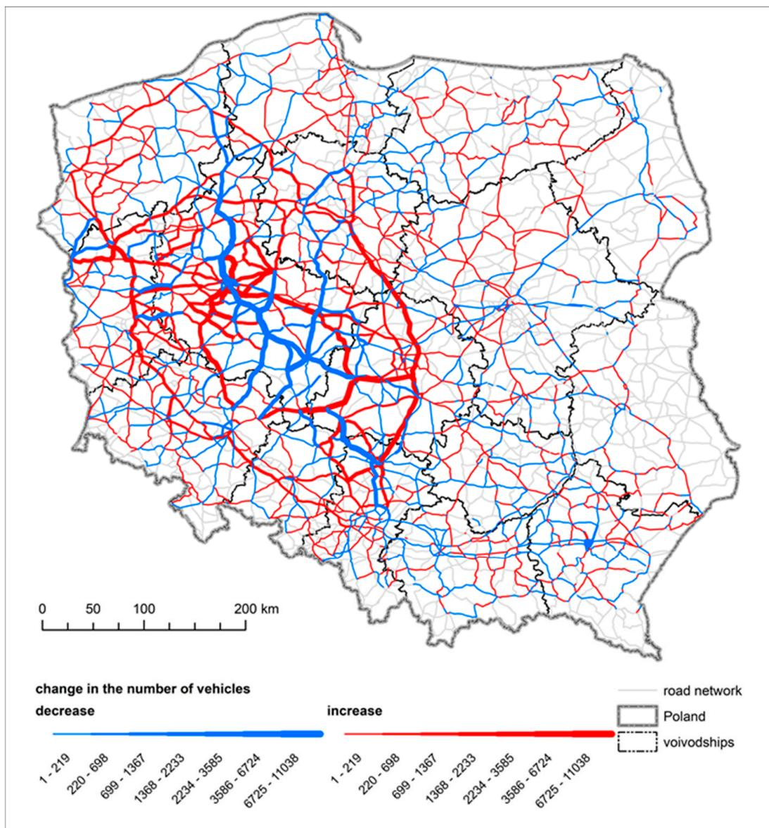
**Figure 5.** Spatial differentiation of vehicle flows for real-time traffic for all trip motivations in the event of a one-hundred-year flood within the Warta Water Region. Source: The authors' own elaboration.
