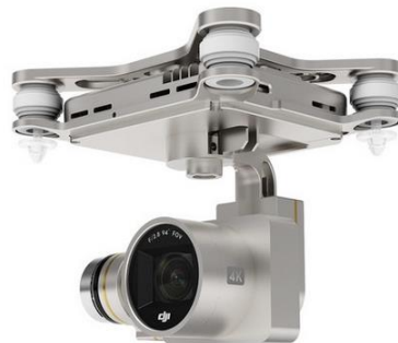
Figure 12. "Sony EXMOR 1/2.3"—4 K" camera mounted on phantom 3 professional.
