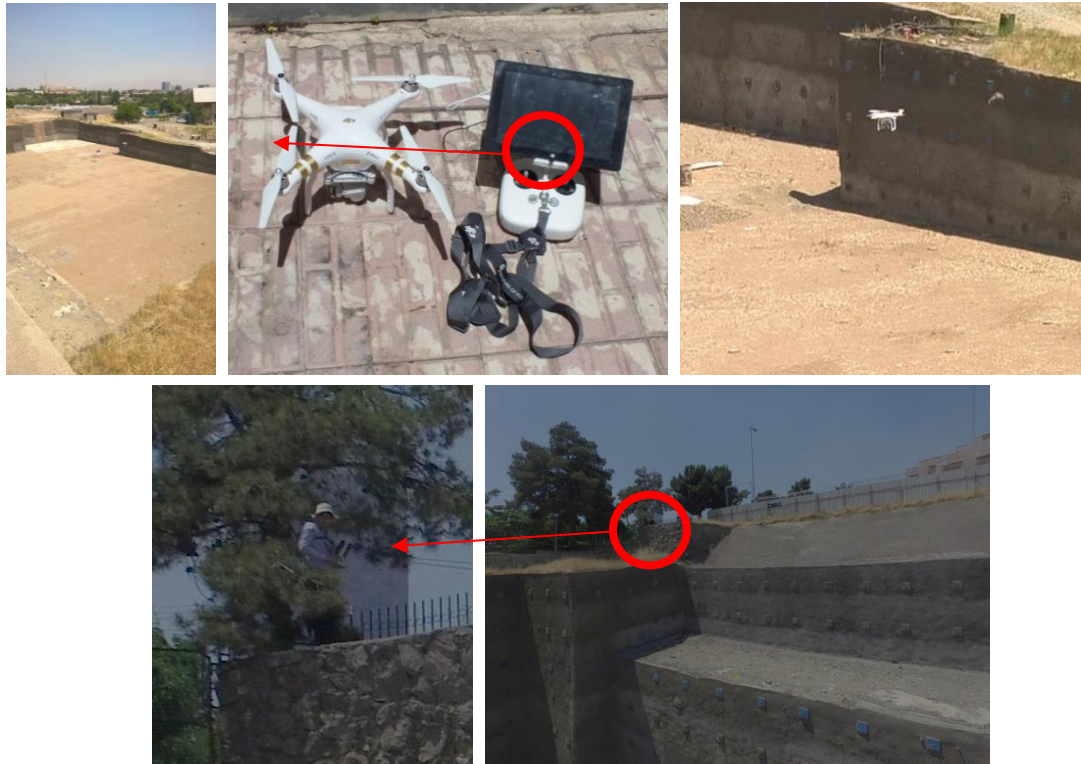
Figure 11. The Phantom 3 Pro when imaging the Seoul excavation pit, along with the drone pilot.
