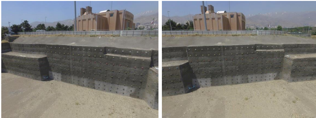
Figure 13. Sample observations captured using the Phantom 3 Pro for displacement monitoring of the excavated wall.
