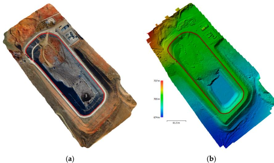
**Figure 4.** (a) Outer boundary on the tiled model; (b) outer boundary on the corresponding DEM.
