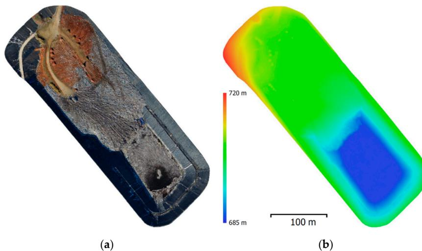
**Figure 5.** (a) Clipped tiled model which includes only the storage area; (b) clipped DEM corresponding to the clipped tiled model.
