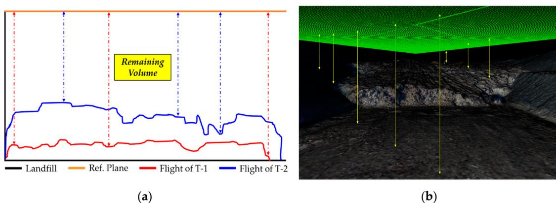
**Figure 7.** (a) Theory of volumetric calculations for the remaining volume; (b) 3D visualization of the volumetric calculation.
