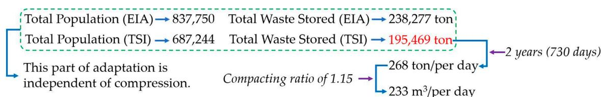
**Figure 8.** Obtaining per-day volume value by using statistical values in the comparison.
