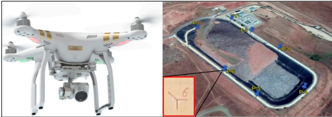
**Figure 3.** The unmanned aerial vehicle (UAV) employed (left) and the distribution of GCPs on the road surrounding the landfill (right).
