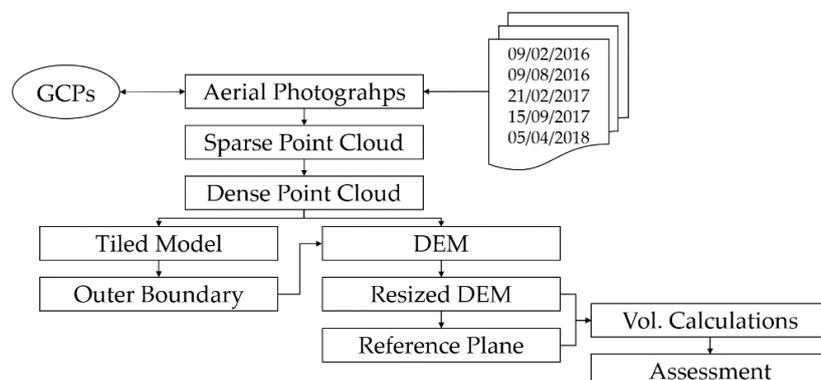
**Figure 2.** Applied methodology involving integration of ground control points (GCPs) with photographs and production of digital elevation model (DEM).
