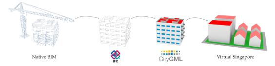
**Figure 1.** The project in a nutshell: from native BIM (Building Information Model) to the integration of CityGML models in Virtual Singapore.
