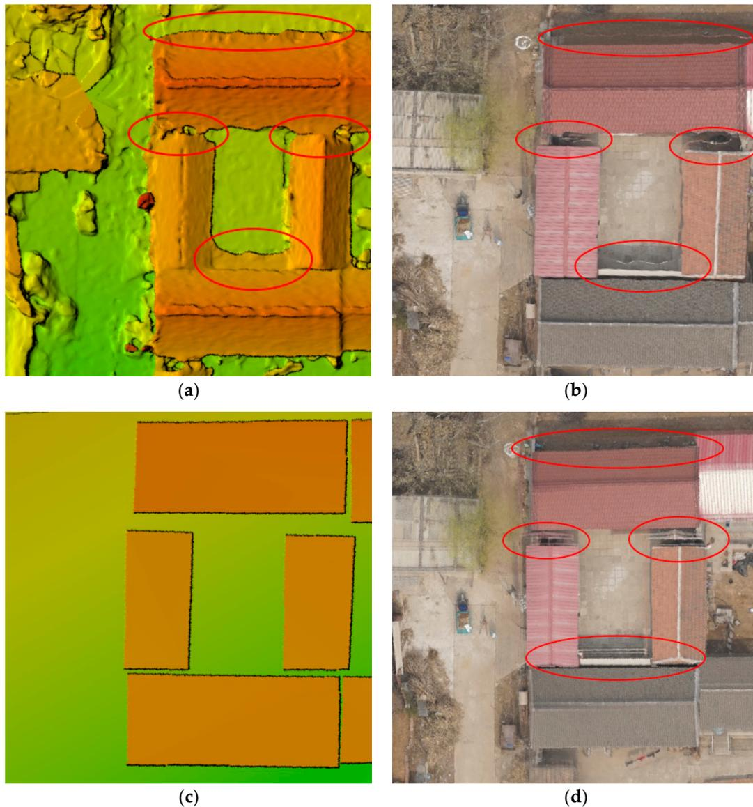
**Figure 7.** (a) Original DSM; (b) original DOM; (c) revised DSM; and (d) the DOM generated by the revised DSM.
