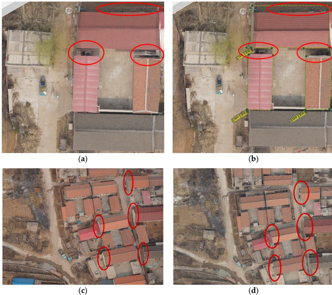
**Figure 8.** (a) Original DOM of the test area A; (b) TDOM of the test area A after multi-view image compensation; (c) original DOM of the test area B; and (d) TDOM of the test area B after multi-view image compensation.
