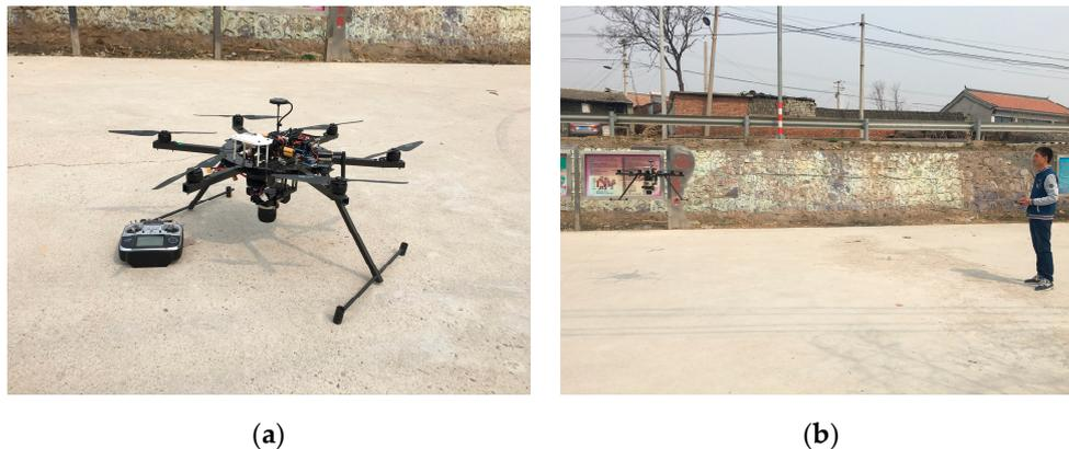
**Figure 3.** Photographs of (a) the DJI S900 UAV equipped with Sony A7r camera and (b) the UAV taking off.
