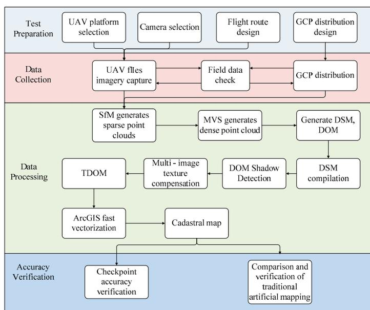
Figure 1. Workflow schematic of the study.
