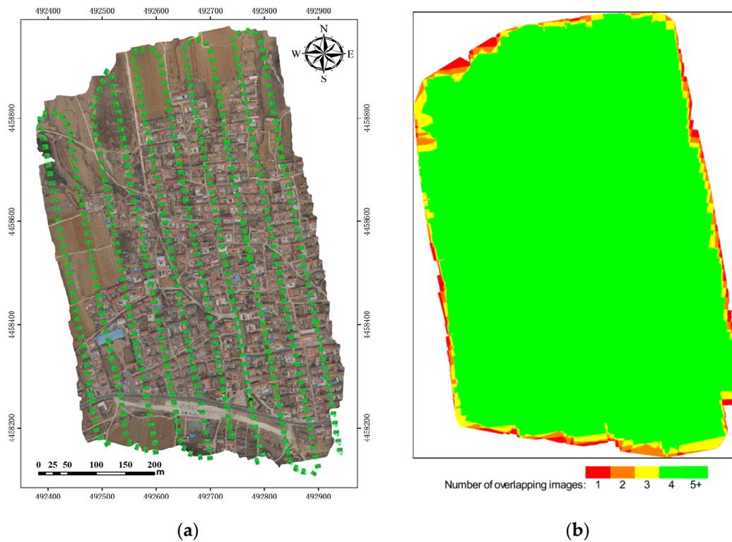
**Figure 6.** Images showing (a) restoration of the camera exposure location and UAV trajectory using the SfM algorithm and (b) the overlap of the digital orthophoto map (DOM) with the UAV point cloud; areas masked in green indicate an overlap of more than five images.
