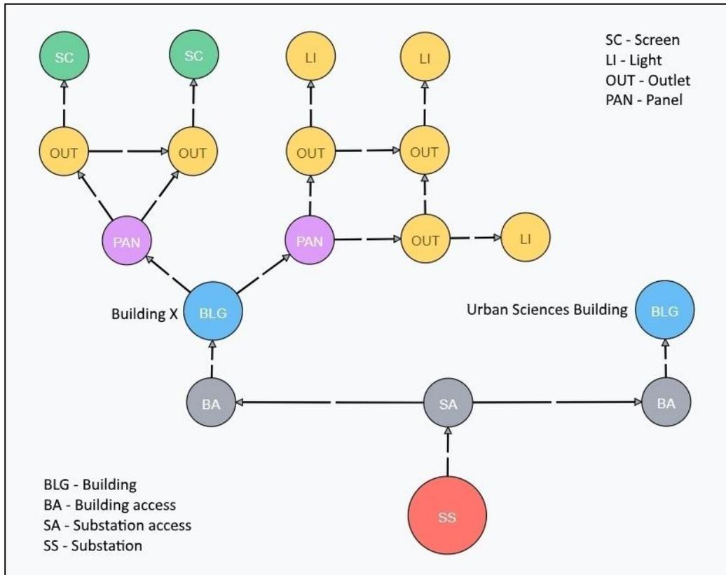
**Figure 6.** The integrated topology of the electricity distribution network highlighted in Figure 2 and the internal electrical components of Building X, as shown in Figure 3.
