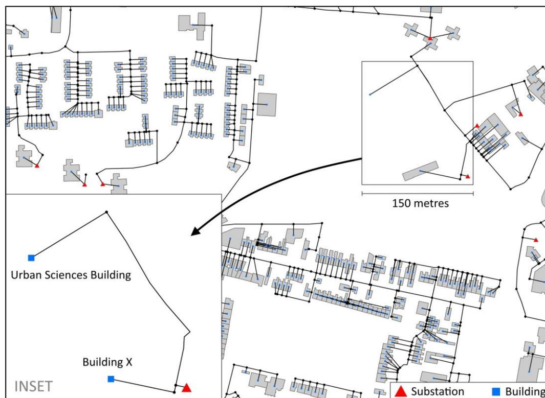
**Figure 2.** Heuristically derived electricity distribution feeder networks for an area of the city of Newcastle upon Tyne, UK. The inset zooms in on a single, small distribution feeder network (located in the top-right of the figure) that is used as the subject network for this study. *Contains OS data © Crown copyright and database right (2018).*
