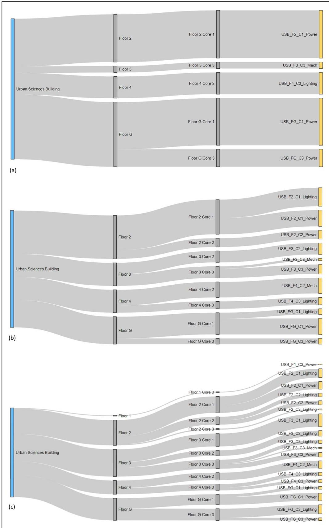
**Figure 11.** Three snapshots, with a time-lapse of approximately 5 s, of an evolving visualisation of the flow of electricity through the Urban Science Building from state (a) to (b) and then (c); in real-time, the visualisation is updated each second.
