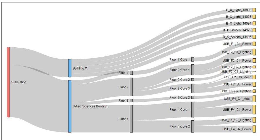
**Figure 10.** Screenshot of a dynamic Sankey diagram, showing electrical power consumption through the network depicted in Figure 7. The thickness of the lines is proportional to the power consumption.
