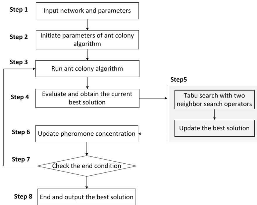
**Figure 3.** Overview of the hybrid optimization algorithm.
