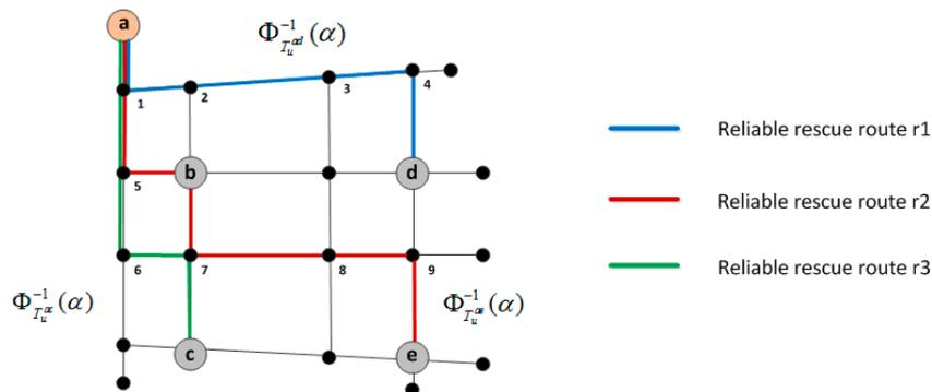
Figure 2. Example of  $\alpha$ -reliable rescue routes from warehouse to affected areas.
