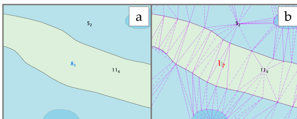
Figure 5. An example of the presence of a survey sounding in a flat triangle. In the pane (a), an 8.3-m survey sounding (in blue) is surrounded by the nodes of a 10-m depth contour that are closer than the charted soundings (in black). As such, the survey sounding will be contained by a flat triangle (that is, with three vertices having a 10-m depth) shown in magenta in the pane (b). By adopting the sounding-in-specific-feature test, the algorithm flagged the survey sounding as a potential discrepancy (shown as grey circle with a depth difference of 1.7 m in red) since it was detected as contained by a depth area with a valid depth range between 10 and 20 m.
