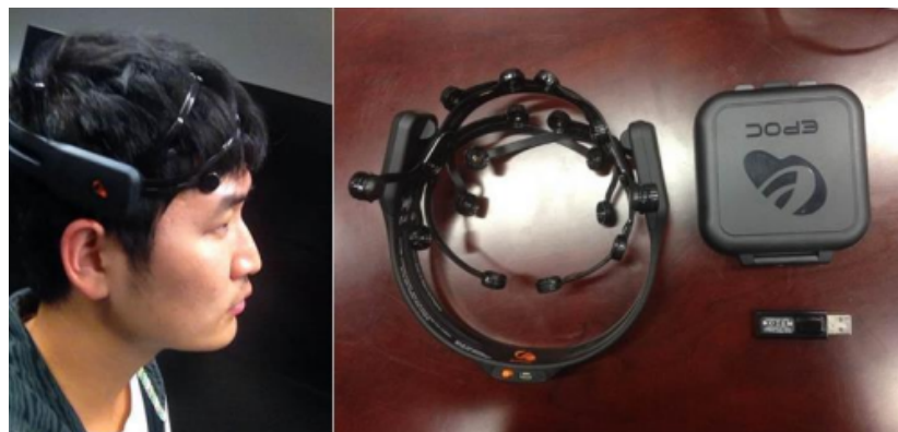
Figure 12. EMOTIV mobile neuroheadset for measuring an individual's brain activities in virtual cognitive experiments.
