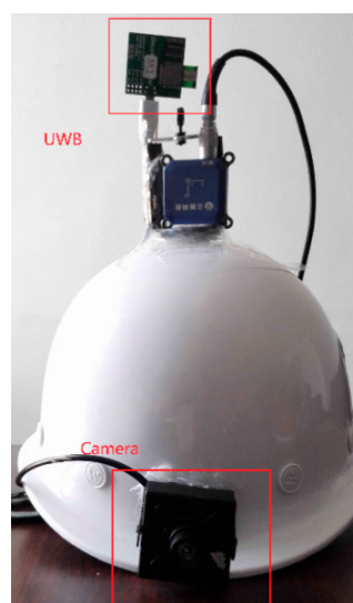
Figure 7. Installation of camera and tag.
