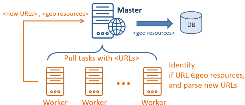
Figure 5. Architecture of distributed computing implementation.
