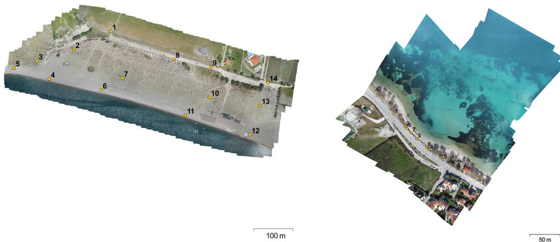
**Figure 5.** The ground control points (GCP) distribution for Eressos beach (left) and Neapoli beach (right).
