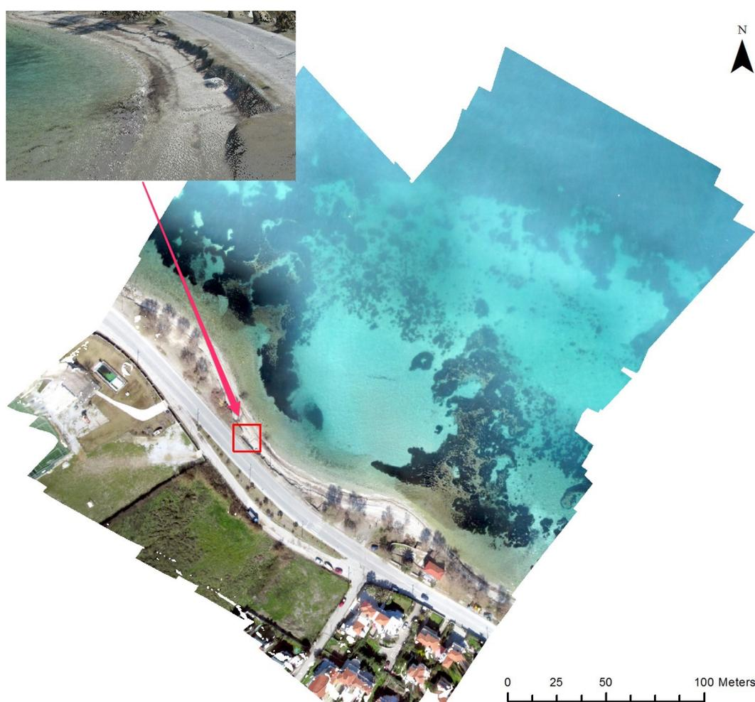
**Figure 6.** The Neapoli study site orthophoto had a spatial resolution of 3 cm. The inset depicts the 3D visualization of the swash zone, wrack lines, and berm zone.
