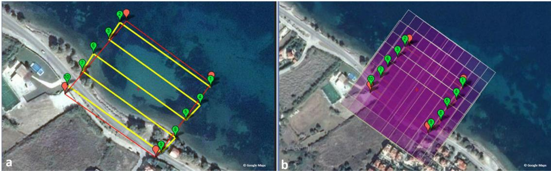
**Figure 3.** (a) Neapoli beach showing the UAV survey lines. The green pointers depict the route followed by the unmanned aerial systems (UAS) (order in-track) and the red pointers depict the four corners of the study area (mission block) (b) The overlap in-track and cross-track sidelap for image acquisition. The purple color depicts the acquired image footprint. (Map data: Google, DigitalGlobe).
