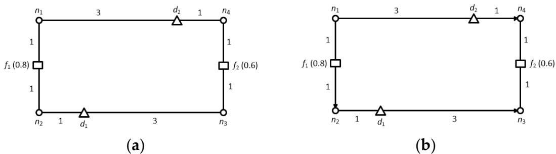
**Figure 8.** Examples (a) undirected road network; (b) directed road network.
