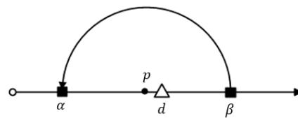
**Figure 5.** Determination of  $\maxdist(d, \vec{\alpha}\beta)$  when  $d \in \vec{\alpha}\beta$ .
