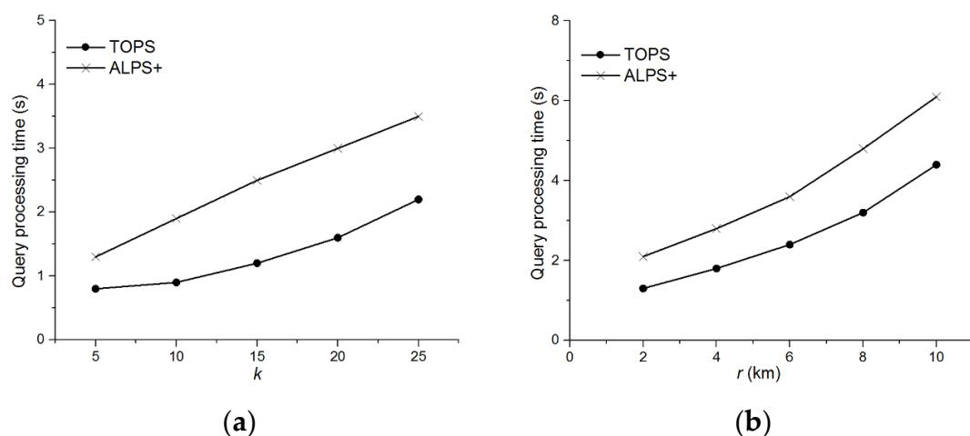
**Figure 16.** Comparison of TOPS and ALPS<sup>+</sup> for  $\theta = \text{rng}$ . (a) Effect of  $k$  on query processing time; (b) Effect  $r$  on query processing time.
