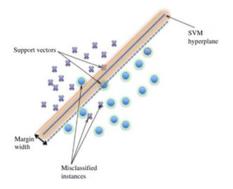
Figure 3. Linear support vector machine example.
