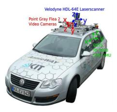
Figure 6. The sensor configuration on the platform (courtesy of [25,26]).
