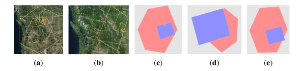
**Figure 14.** (a) Hexagonal cells of the PYXIS framework at several successive resolutions; (b) corresponding cells of (a) in Cube (one-to-four); (c,d,e) PYXIS cells at resolution three, six and seven and the corresponding cells in Cube (one-to-four) at resolution four, six and seven. Cells are uniformly scaled to provide better visualizations.
