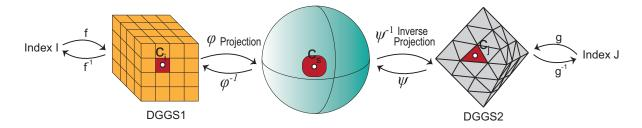
**Figure 11.** Index I in Discrete Global Grid System 1 (DGGS1) is mapped to the refined polyhedron by mapping f. The cell is then projected to the sphere by the projection  $\varphi$  used in DGGS1. Then, the centroid of cell I is inverse projected by the inverse projection  $\psi^{-1}$  of DGGS2. The index J in DGGS2 is then found using inverse mapping  $g^{-1}$ .
