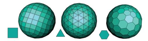
Figure 3. Quadrilateral, triangular and hexagonal cells on spherical polyhedrons.
