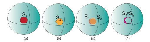
**Figure 13.** (a)  $S_1$  is the subset of points on the sphere enclosed by DGGS1; (b)  $S_2$  is the subset of points on the sphere enclosed by DGGS2; (c)  $S_1$  and  $S_2$  are overlapped (d) The error is  $S_1 \oplus S_2$ , which is the difference of the areas that are enclosed by  $S_1$  and  $S_2$ .
