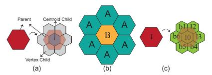
**Figure 6.** (a) A coarse cell (red) is refined to finer cells. Children are categorized as vertex and centroid children. (b) Type Bcells are surrounded by type Acells; (c) the children of a cell with index Iget indices I0to I6 based on their position relative to their parent.
