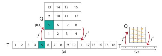
**Figure 7.** (a) Function f maps parameters on T to domain Q. For instance, t = 5 is mapped to [0,1]. Parameters on T are used as indices of Q. (b) A space filling curve that performs row major traversal is illustrated in orange.
