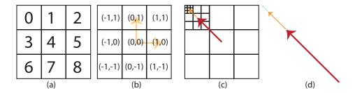
**Figure 12.** (a) Indices in the hierarchy-based indexing method used in SCENZ-grid and (b) the corresponding integer indices for each digit of (a) based on the defined coordinate system; (c) vectors corresponding to index I000; (d) magnified vectors from (c) for a better illustration.
