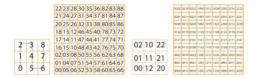
**Figure 15.** (**Left**) Indexing of quadrilateral one-to-nine refinement at two successive resolutions using the Peano SFC with base nine; (**Right**) the same indexing, but with base three.
