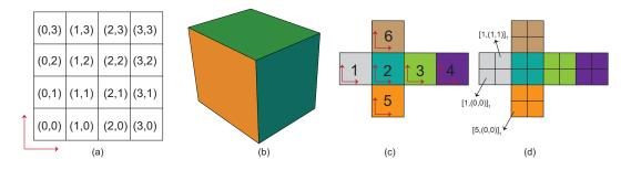
**Figure 10.** (a) Integer indexing of cells using Cartesian coordinates; (b) a cube; (c) the unfolded cube in (b) and coordinate systems for each face; (d) indices of some cells after one step of one-to-four refinement.
