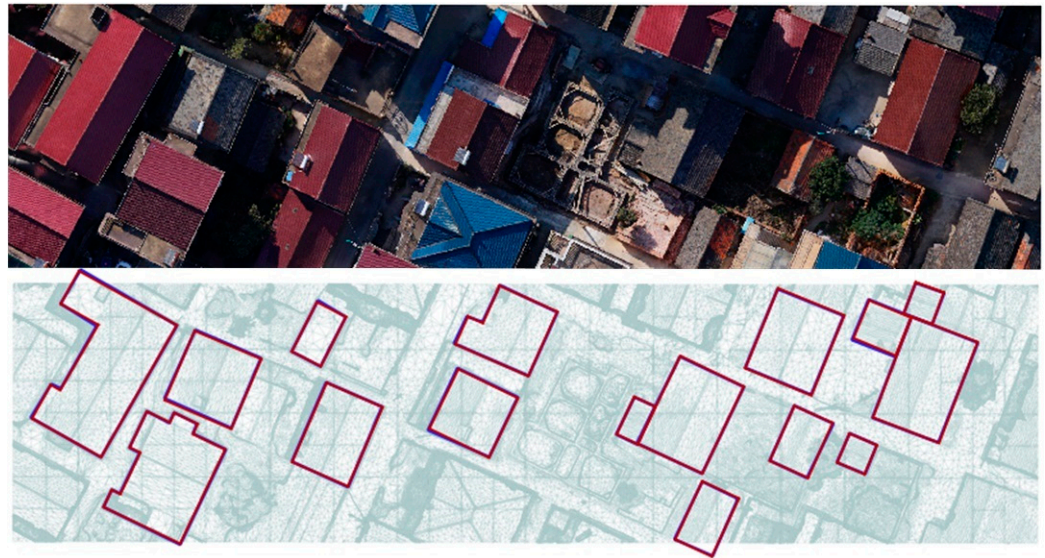
Figure 9. Extraction results of Dataset-1. Red outlines are extracted results and blue outlines are reference data.
