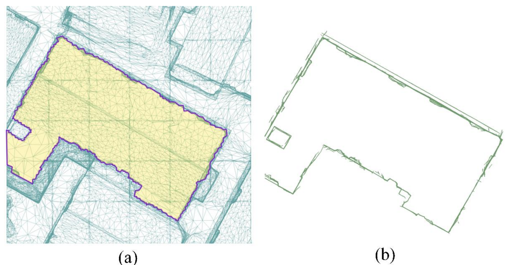
Figure 4. Selecting triangular facets data of outer walls based on roof extent: (a) generation of the bounding polygon (purple) derived from the selected roof grid; (b) identification of potential triangular facets of outer walls using the bounding polygon.
