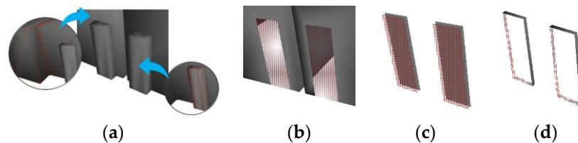
**Figure 8.** Intersection (a), room solid with opening (b), boundary surface (c), door solid with opening (d).
