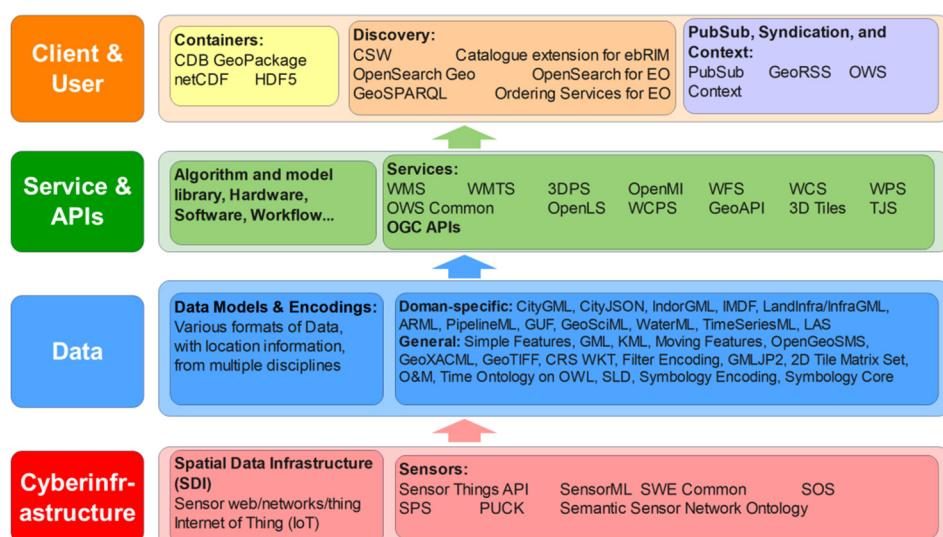
**Figure 1.** Functional architecture of OGC implementation specifications.
