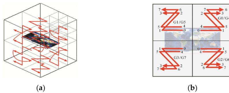
**Figure 4.** Schematic diagram of the coding sequence of GeoSOT 3D grid cells [26]. (a) Oblique view; (b) Top view.
