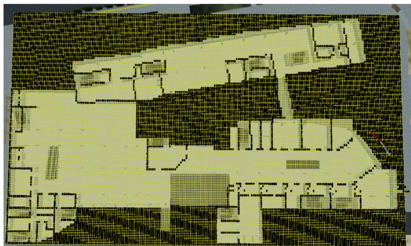
Figure 14. BIM model analysis to generate indoor grid topology map.
