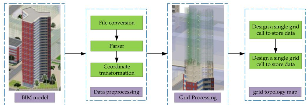
**Figure 5.** Indoor grid map construction process.
