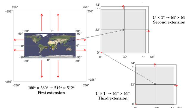
Figure 2. GeoSOT mesh three expansion process [25].
