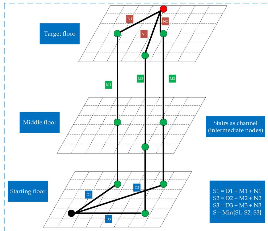
Figure 10. GeoSOT-A\* Algorithm Path Planning Display.
