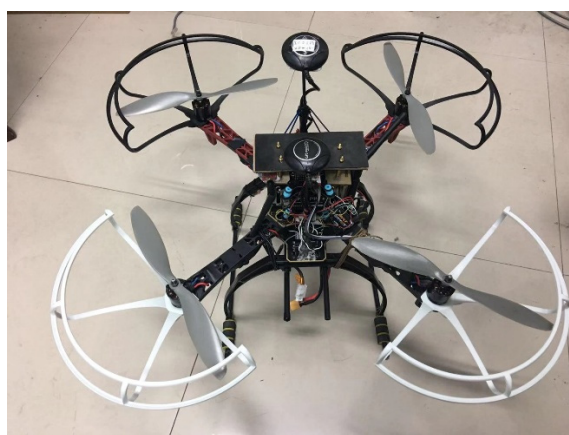
Figure 13. The self-designed four-rotor platform.
