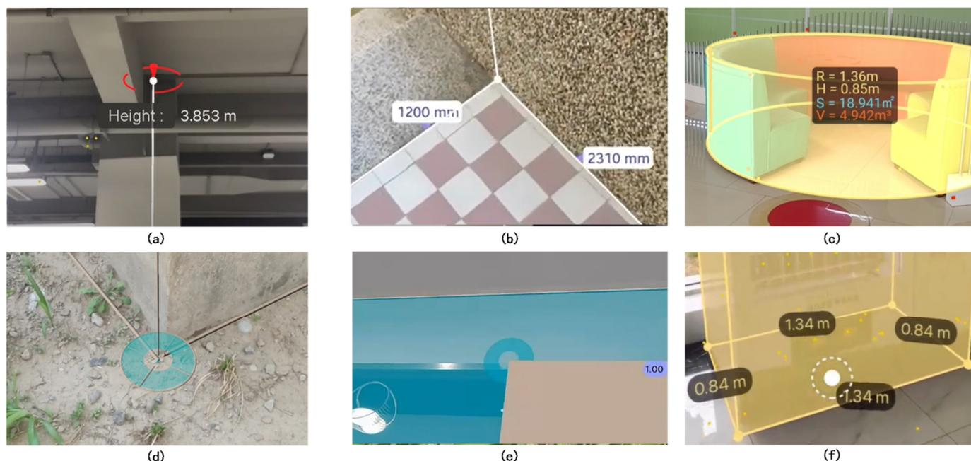
**Figure 10.** Modeling visual view of buildings in ARSnap: (a) Display the elevation line snap results of the real scene, (b) display the vector snap results of the virtual scene; (c) display the snap results of the irregular sofa; (d) display the plane snap results of the real scene; (e) display the wall snap results of the virtual scene; (f) display the snap results of the regular vending machine.
