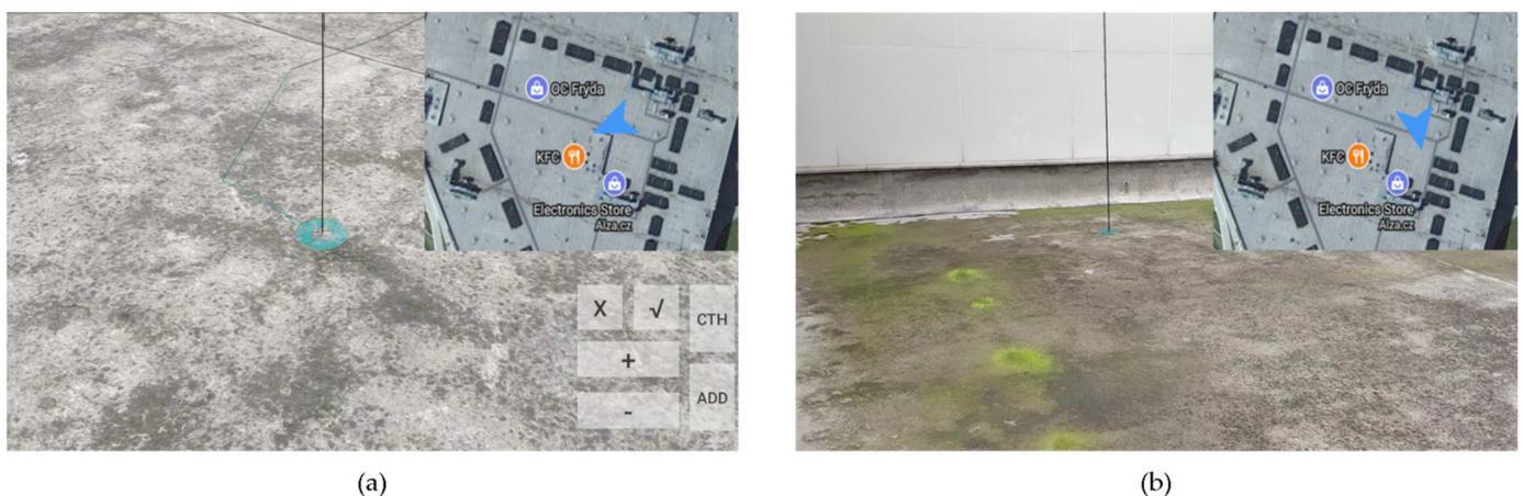
**Figure 11.** Capturing points on the specified 3D plane: (a) snapping to a point in a 3D plane (short distance); (b) snapping to a point in a 3D plane (far distance).
