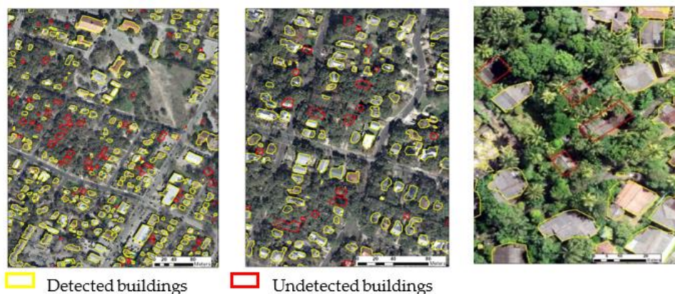
Figure 17. Undetected buildings due to being covered by trees.
