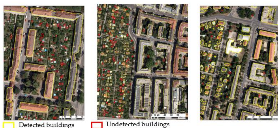
Figure 16. Undetected buildings from the proposed model due to the building size becoming minor.
