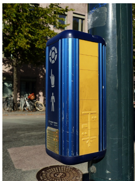
Figure 2. A simple tactile map by a pedestrian crossing in the city of Trondheim (source: authors).
