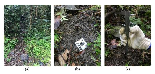
**Figure 2.** Illustration of field measurements in the Shihmen Reservoir watershed: (**a**) a natural slope, (**b**) an erosion pin and its label, and (**c**) measuring with a caliper ((**c**) from [22]).
