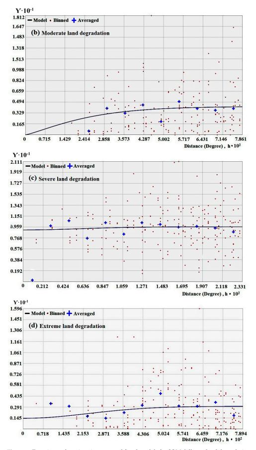
Figure 2. Experimental semi-variograms and fitted models for SOM different land degradation types.
