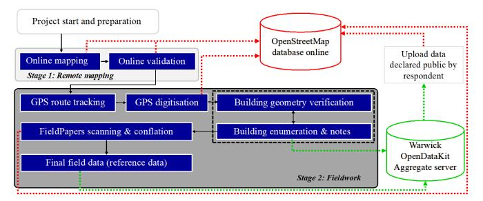
Figure 1. Participatory mapping process workflow with defined stages in grey background.
